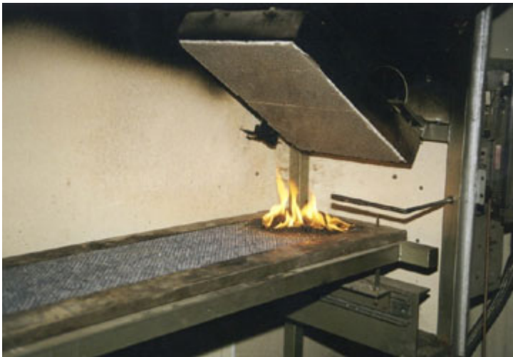
A photo of a floor covering being fire tested to the requirements of ISO 9239.1
